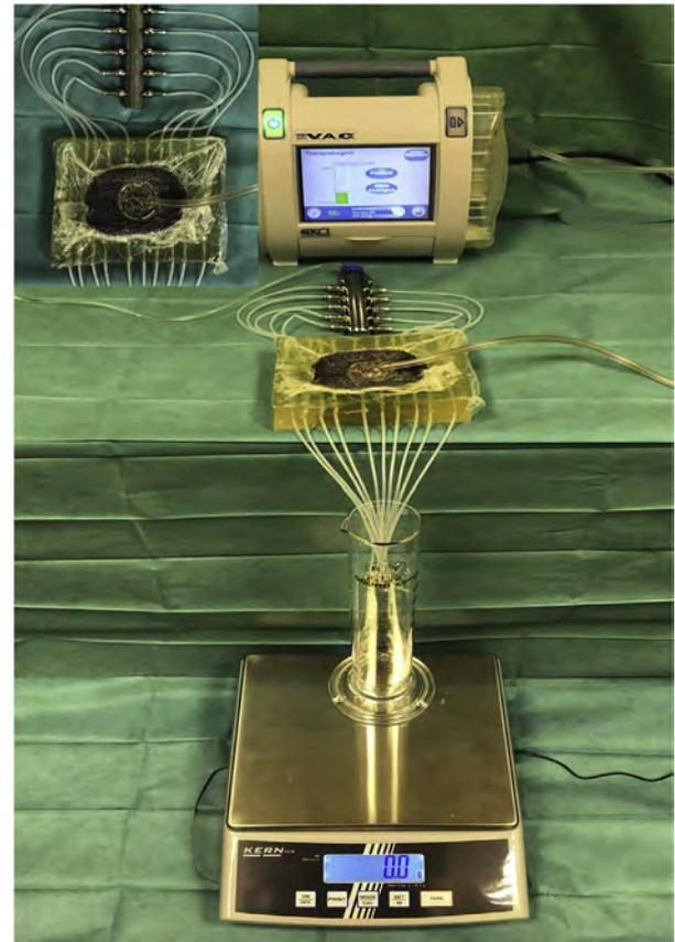
Fig. 2. Perfusion test with multiple rubber tubes embedded in a block of 300 bloom ballistic gel (Type A, TMP-products, Bad Camberg, Germany) covered by a standard NPWT system. The efferent tube endings lead into a collecting cylinder on a gauged electronic scale.
