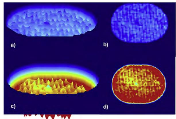
Fig. 3. Three (a and c) and two-dimensional (b and d) and pressure profile of the entire surface area of the foam (75 cm<sup>2</sup>). Centrally, in close proximity to the trackpad is an area of significantly lower positive pressure.
