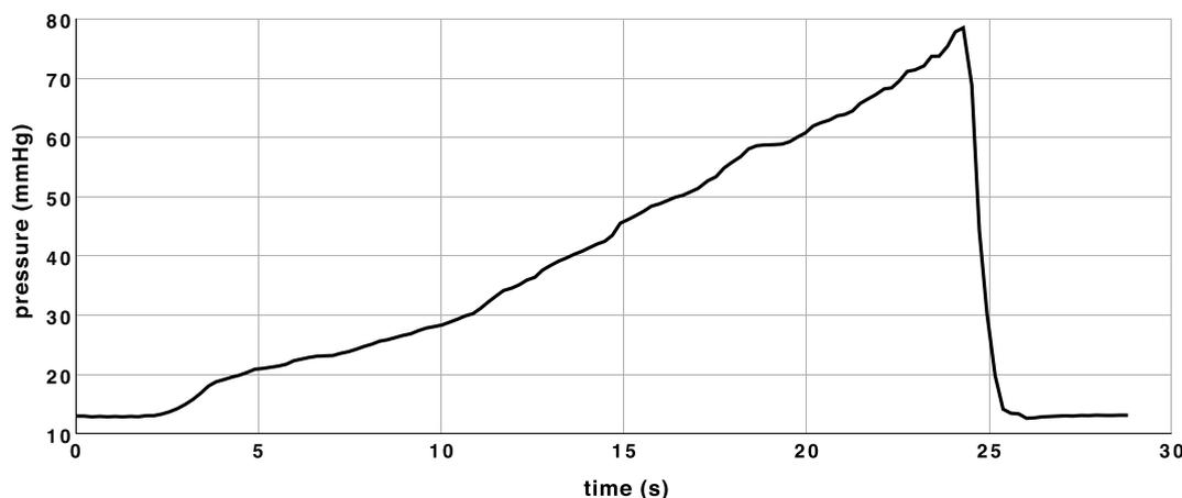
Fig. 6. Rise in average pressure up to a maximum of 78 mmHg (1.04 N/cm<sup>2</sup>) at 125 mmHg of vacuum.
