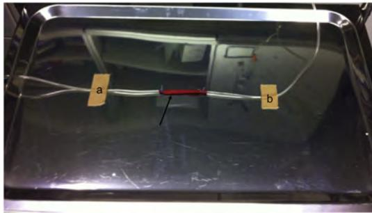
Fig. 1. Perfusion test using single vessel imitation (arrow) with afferent (b) and efferent (a) tube before covering with a standard NPWT system.
