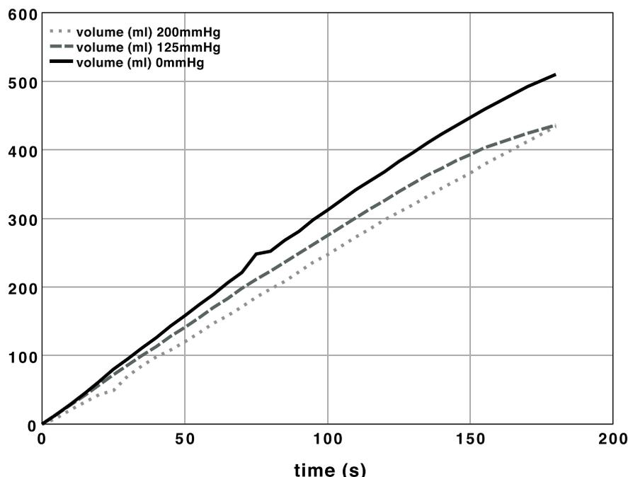
Fig. 5. Results of the perfusion test using ballistic gel. A significant difference between 125 mmHg (dashed line) and 200 mmHg (dots) of suction pressure was found in comparison to baseline flow (solid line).
